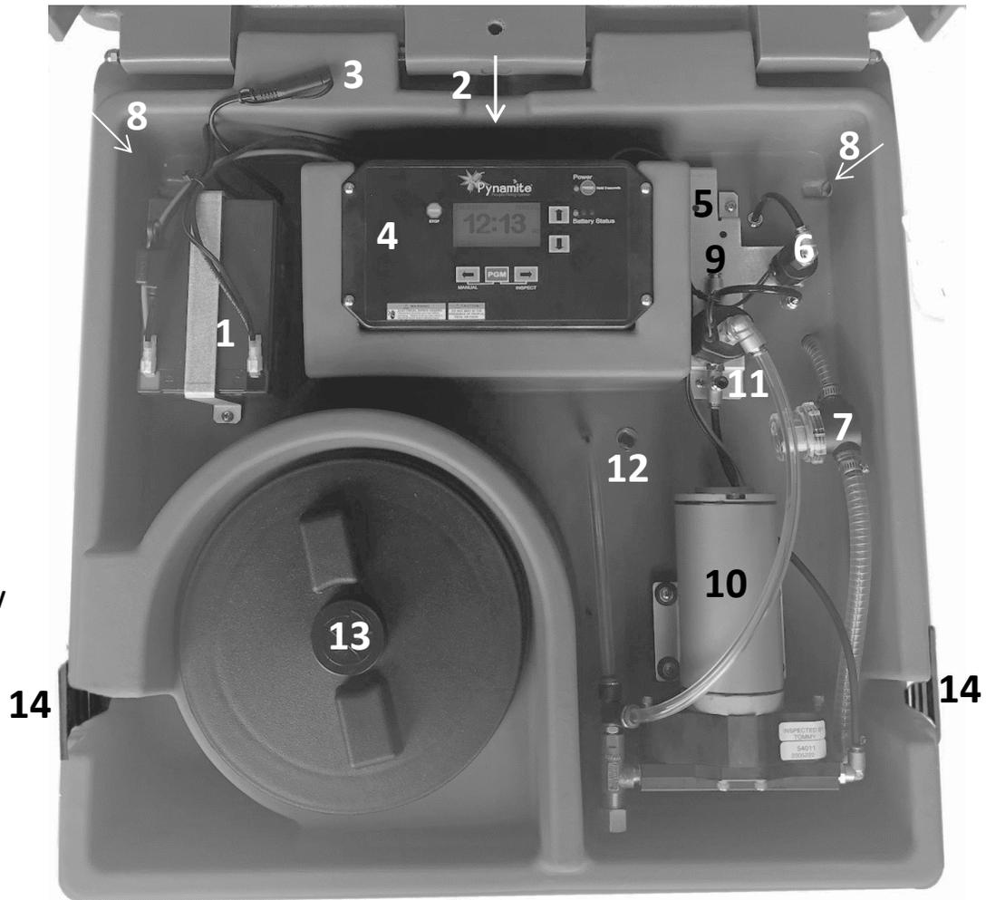
1. BATTERY - Connects to the Controller and Battery Charger.
